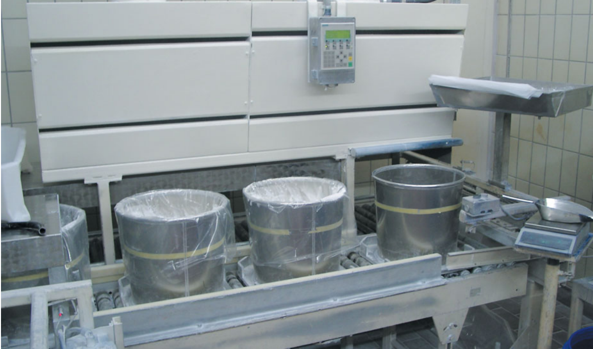
At EVC, as many as twelve different additives are now weighed PC-based in accordance with a recipe and then placed in bags
