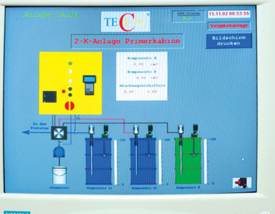
Even the mixing of two-component coatings, although previously conventionally controlled, has become part of PC-based Automation at Teclac
